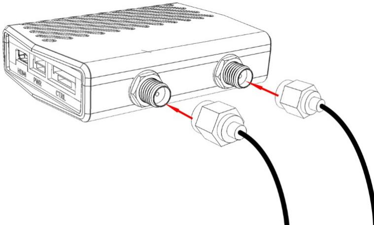
Connecting the Antennas to the Air Unit
