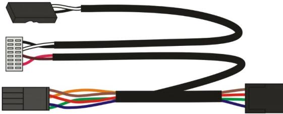
The middle connector of this cable goes into the Air Unit CTRL port.
