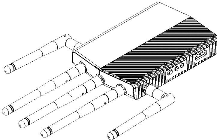
Connecting the Ground Unit Antennas – Box 4
