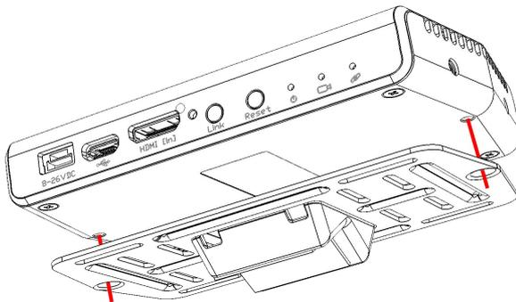
Attaching the Air Unit to the Mounting Plate
