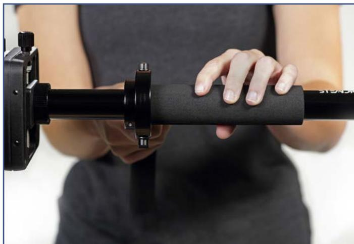
**Release the Post and observe how fast the SOLO drops.**
