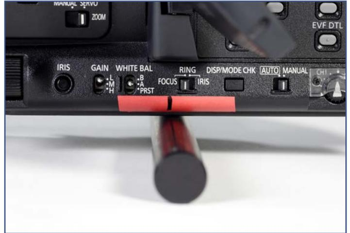
Rotate the camera 90° and find the **Side-to-Side** balance point.
