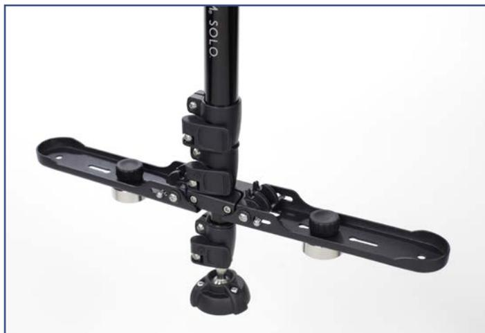
Remember to re-adjust the **SOLO** so it is in **Static Balance** after changing the weights by moving the **Gimbal** or adjusting the length of the **Post**.
