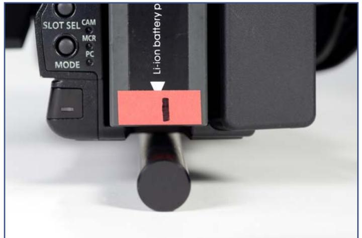
**NOTE:** Some cameras (like DSLRS) may have balance points **OUTSIDE** of the camera body. In that case, you would mount the QR Plate to the camera **FIRST** and use the pen to find and mark the balance points.
