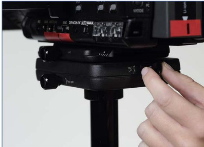
**Continue these adjustments until the Post remains vertical in both axes with a 2 second drop time.**
