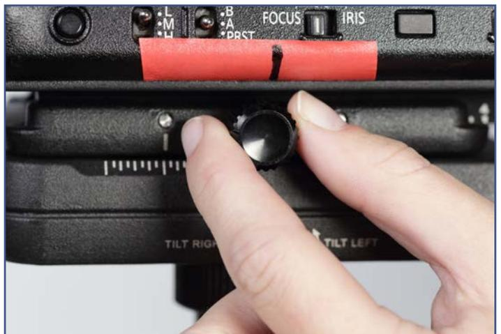
Using the **Side-to-Side Adjuster Knob**, align your **Side-to-Side** mark with the **CENTER** of the **Post**.
