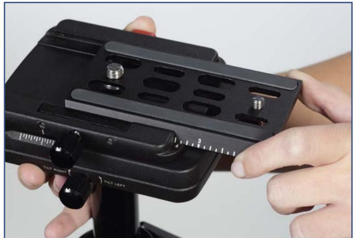
Center the **Camera** to the **QR Plate** by using the **Fore-and-Aft** and **Side-to-Side** marks you made.
