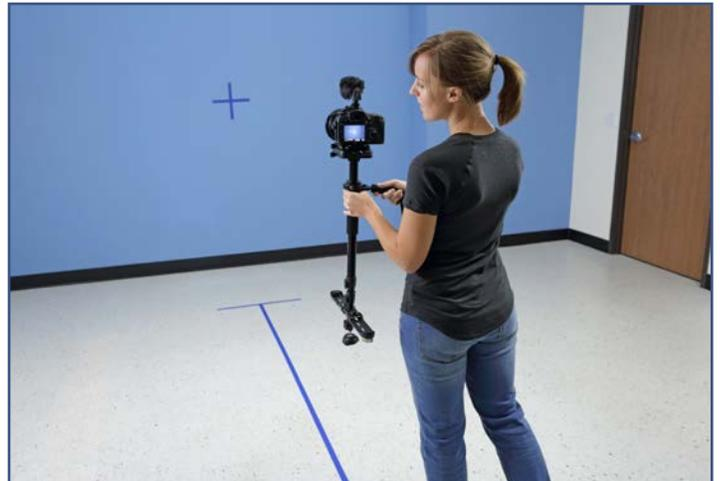
Walk forward and backwards with the frame centered on the crosshair. Concentrate on maintaining a level horizon, the camera shouldn't look like you're on a boat!
