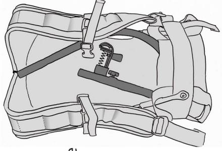
How to fold the arm correctly into the bag.
