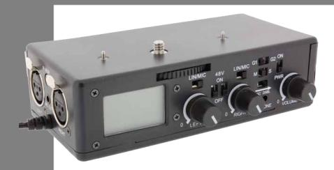
The BeachTek DXA-5D is a two-channel, transformer balanced XLR adapter for attaching external microphones and other audio gear to the Canon 5D Mark II camera. It can also be used with any camcorder or other audio recording device that has a built-in mic jack.
